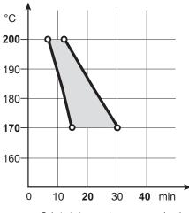
Substrate temperature versus curing time
