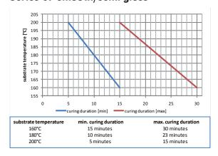
Please observe cure parameters closely since mechanical properties will develop before full cross-linking!
